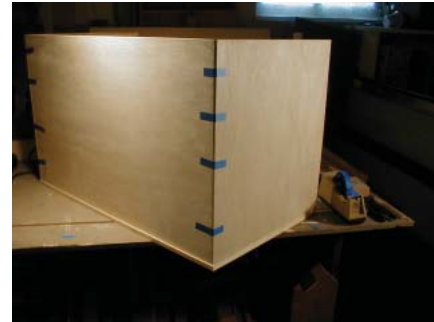
Use masking tape to secure panels while the glue sets.
