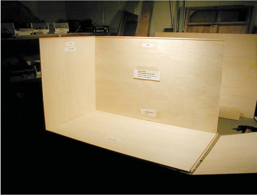
Use masking tape to secure panels while the glue sets.
